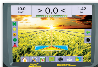
REALVIEW GUIDANCE OVER VIDEO; GUIDANCE CAN BE TURNED OFF AT ANY TIME
