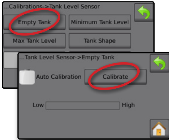
Figure 33: Tank Level Sensor – Empty Tank
